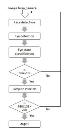
Fig. 3. Perclos computation framework
